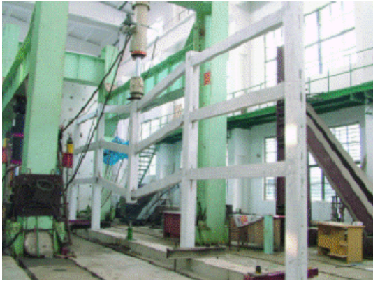
Fig. 5 Collapse test of plane frame
